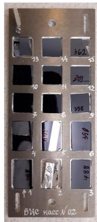
**Figure 2.** Photo of a holder cassette with several heterostructures.
