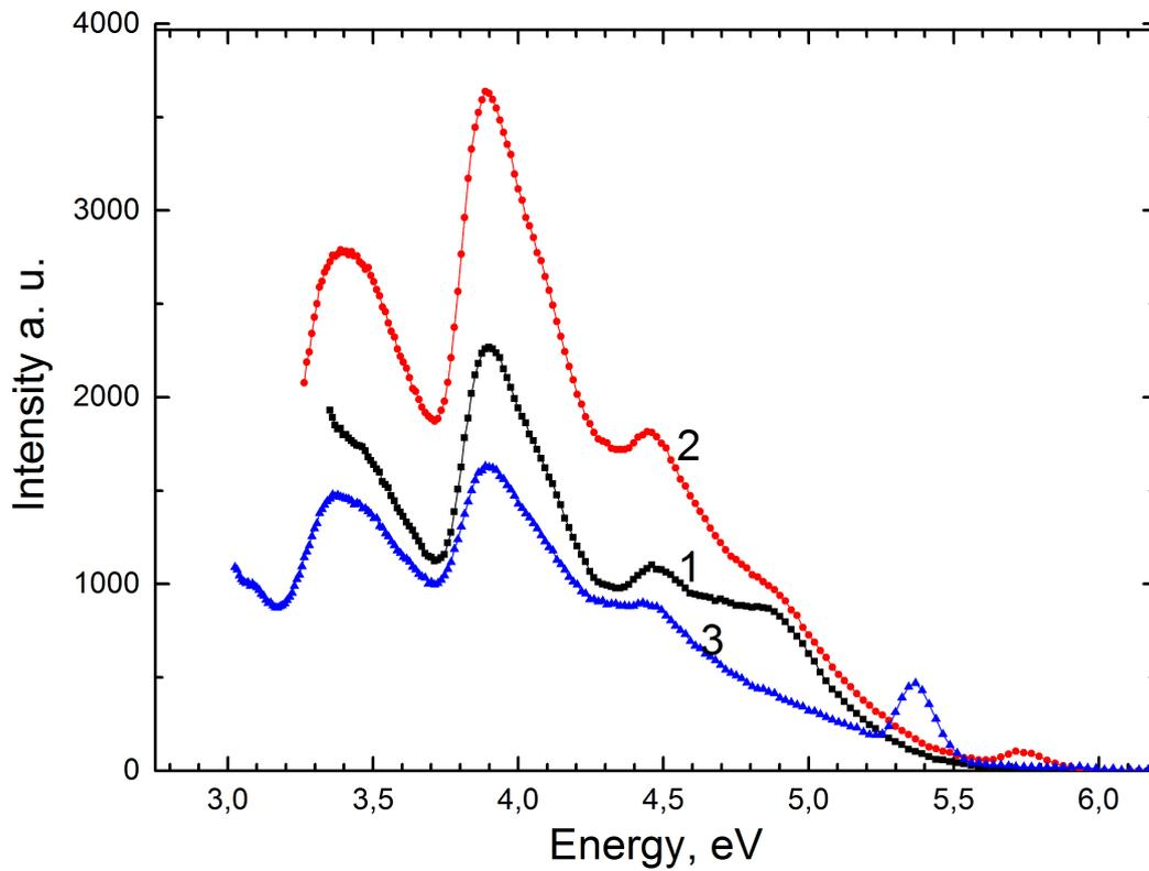
Figure 3. Excitation spectrum  $\text{Li}_2\text{SO}_4\text{-Cu}$  for emission bands 1-3,18 eV, 2-3,05 eV, 3-2,84 eV at 80 K.
