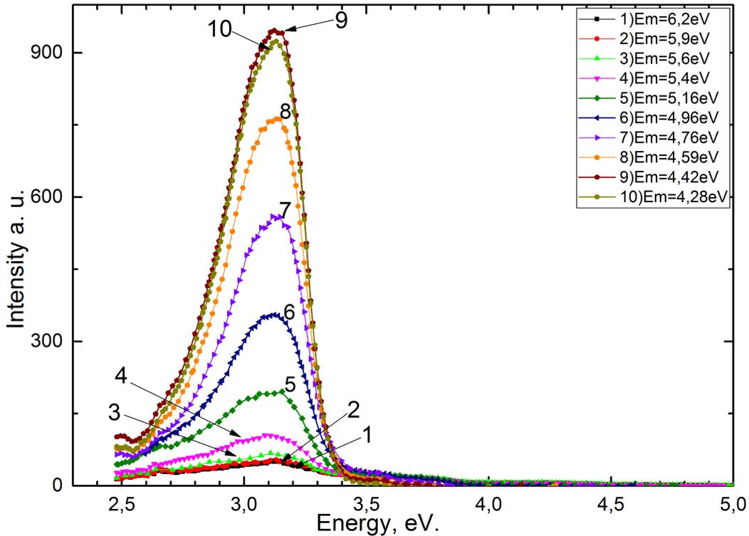
Figure 4. The emission spectra of X-ray irradiated  $\text{Li}_2\text{SO}_4\text{-Cu}$  crystal at the excitation by photons from 4.27 eV to 6.2 eV at 80 K.
