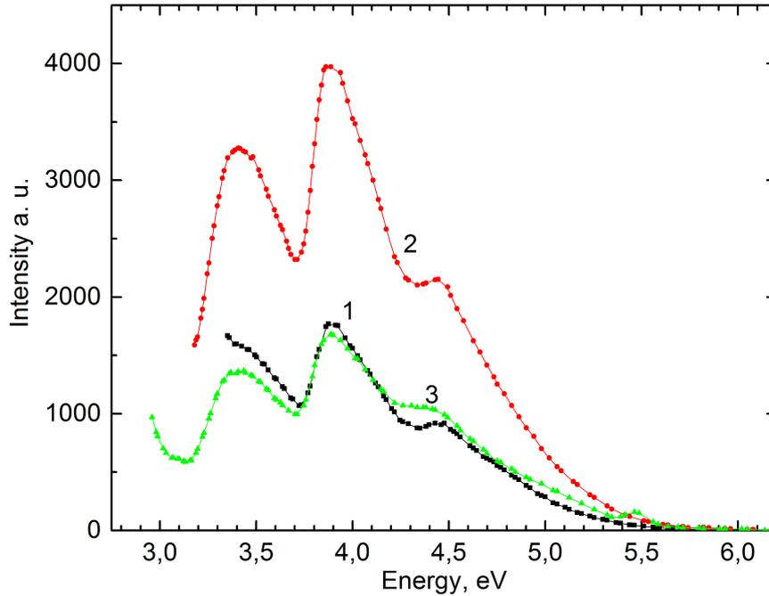
Figure 5. Excitation spectrum of X-ray irradiated crystal  $\text{Li}_2\text{SO}_4\text{-Cu}$  : 1-3.18 eV, 2-3.05 eV, 3-2.84 eV at 80 K.
