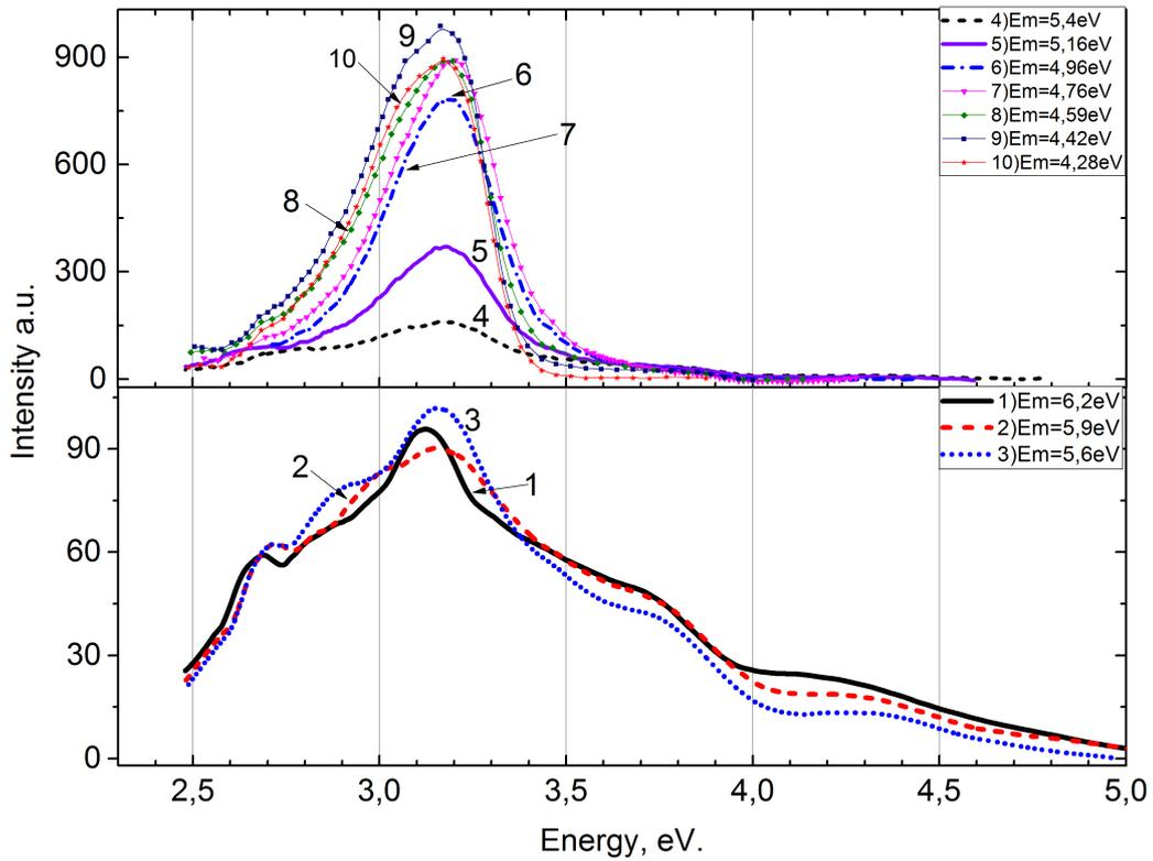
Figure 2. Emission spectrum of highly pure (99.99%) powder  $\text{Li}_2\text{SO}_4\text{-Cu}$ , when excited by photons with an energy from 4.27 eV to 6.2 eV at 80 K.
