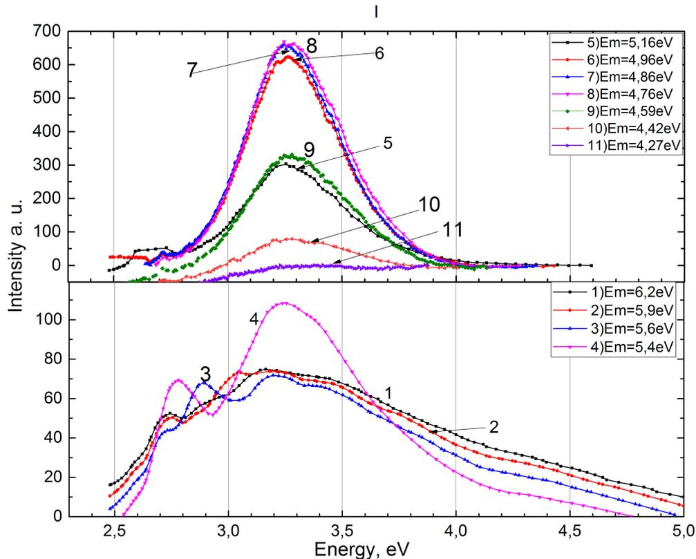
Figure 1. Emission spectrum of highly pure (99.99%) powder  $\text{Li}_2\text{SO}_4\text{-Cu}$ , when excited by photons with an energy from 4.27 eV to 6.2 eV at 300 K
