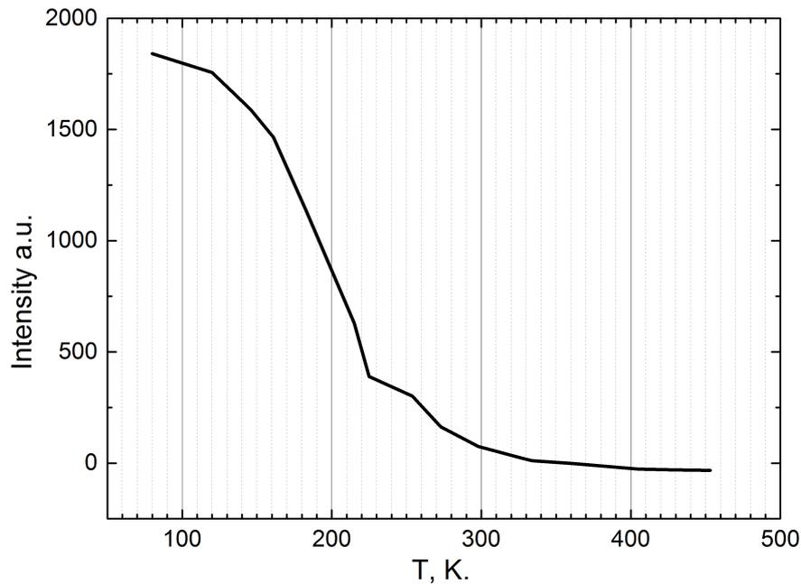
Figure 6. Temperature dependence of the emission band of 3.13 eV of the  $\text{Li}_2\text{SO}_4\text{-Cu}$  crystal irradiated with photons with an energy of 4.77-4.96 eV at 80 K.
