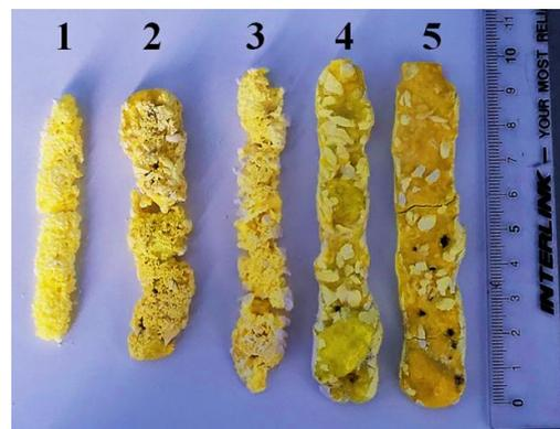
**Figure 4.** Photographs of YAG:Ce ceramic samples synthesized under the influence of electron fluxes of different  $E$  and  $P$ : 1— $E = 1.4$  MeV,  $P = 2.5$  kW/cm<sup>2</sup>; 2— $E = 2.0$  MeV,  $P = 4$  kW/cm<sup>2</sup>; 3— $E = 2.5$  MeV,  $P = 8$  kW/cm<sup>2</sup>; 4— $E = 2.0$  MeV,  $P = 6$  kW/cm<sup>2</sup>; 5— $E = 2.5$  MeV,  $P = 10$  kW/cm<sup>2</sup>.
