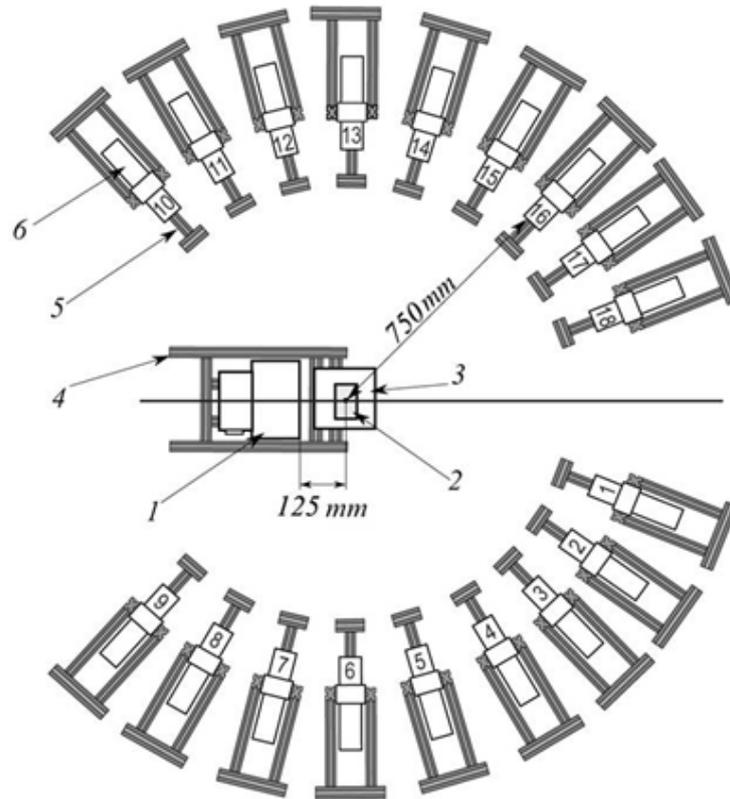
Figure 1. The experimental setup "Romasha": 1 - ING-27 neutron generator; 2 - target; 3 - target holder; 4 - aluminum frame of the setup; 5 - supports for  $\gamma$ -radiation detectors; 6 -  $\gamma$ -radiation detectors; numbered from 1 to 18.
