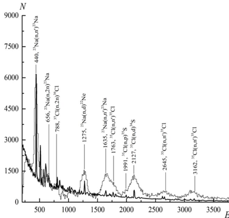
Figure 3. Spectra of  $\gamma$ -emission obtained by irradiation of a NaCl sample with neutrons with an energy of 14.1 MeV. The thin line shows the spectrum measured with the BGO scintillation detector, the bold line - with the HPGe detector. The energies of the revealed  $\gamma$ -transitions are indicated according to ENSDF [10].
